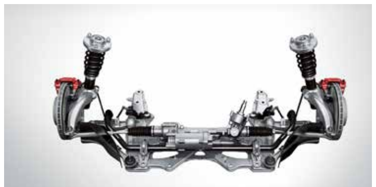
The 2016 Cayman S with its electronic assisted rack and pinion steering system
