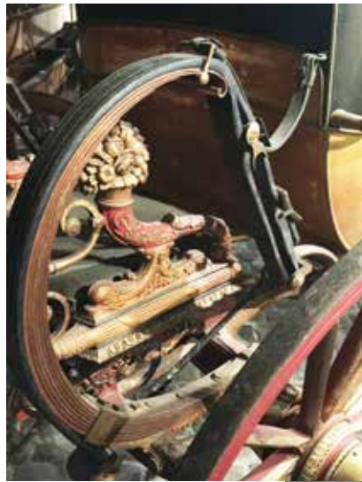
Suspension from the 8 horse power coach at Versailles
