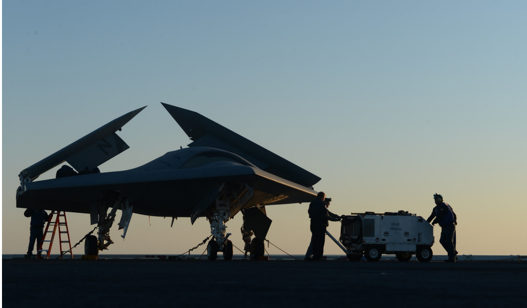
Northrop Grumman personnel conduct preoperational tests on a U.S. Navy X-47B Unmanned Combat Air System demonstrator aircraft on the flight deck of the aircraft carrier USS George H.W. Bush (CVN 77) May 14, 2013, in the Atlantic Ocean.
