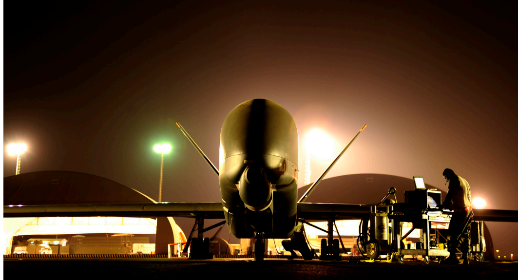
U.S. Air Force maintenance technicians conduct preflight checks on an RQ-4 Global Hawk unmanned aerial vehicle assigned to the 380th Expeditionary Operations Group at an undisclosed location in Southwest Asia Nov. 23, 2010.
