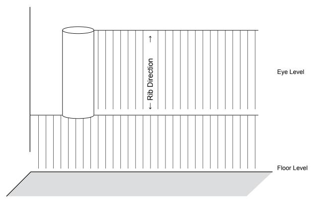
When installing **Prep** on walls with ribs running vertically, run full roll along ceiling line to keep seam below eye level.
