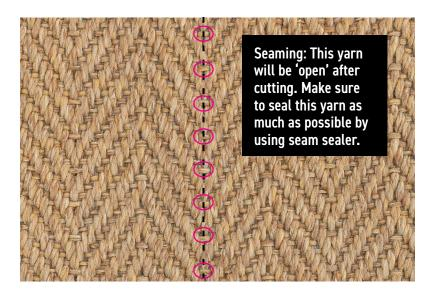
Figure 2: Take care to leave the lower lockstitch on the "good" side of the seam. Score first to open the row. Cut with the outside blade. Seal seams and after the seam is put together, trim with duck-billed sheers.
