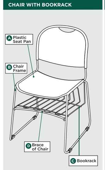
Locate area between Plastic Seat Pan A and Chair Frame B and secure Rear Bookrack Hooks Co to Frame.
