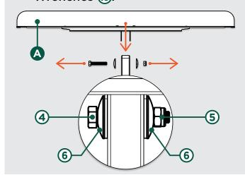
To install the tray B, align holes on the Tray Bracket B with the holes on the Inner Tube D, to secure the Tray in position use the M6x40 screws provided
