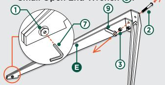
Install Conductor's Base (a) to Telescopic Tube (b) as follows: Begin by Inserting the telescopic tube through the base. Align the two base holes over two holes on telescopic tube. Insert two M6x50 Bolts (2) and tighten with two M6 Lock Nuts (3) using 4.0 Allen Wrench (8) and Small Open End Wrench (9).
