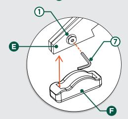
Ensure that all bolts are fastened tightly.
