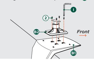
Align the holes on Seat Bases with the holes on Seat Frames . Insert two M8 x 45 Bolts 5 and tighten with two Nuts 6 using Enclosed Hex Key H and Open end Wrench J.
