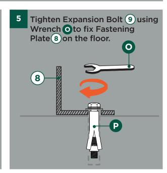
**OPTIONAL FLOOR CONNECTION-ASSEMBLY COMPLETED**
