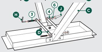
Pon't fully tighten the Bolts until you make sure that the main structure is level with the ground at Step 4.
