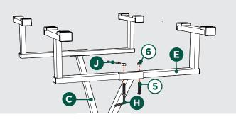
Place Seat B) downward on a flat and clean surface. Note that the arrow on Seat Base B2 should point foward.
