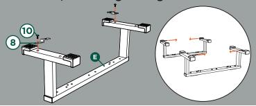
Make sure that four Legs touch the ground evenly and then tighten the Bolts within Step 1 and 2.
