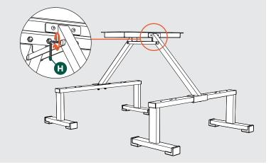
Align the holes on two Connecting Plates D with the holes on two sides of Connecting Frames C. Insert two M8 x 55 Bolts 3 through four Washers 4 and tighten with two Nuts 6 using enclosed Hex Key H and Open End Wrench J.
