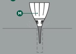
Align the holes on Fastening Plate 8 with the holes on the floor. Knock Expansion Bolt 9 into the hole using Hammer L.
