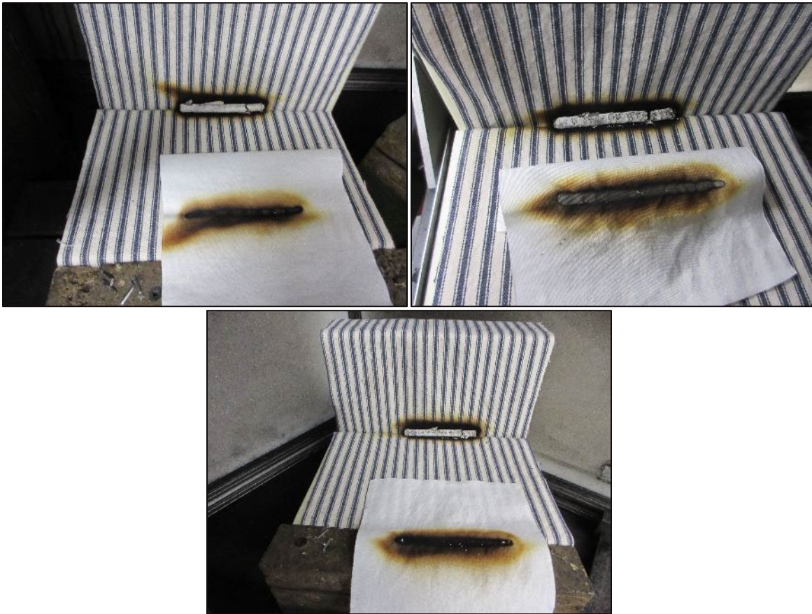
Figure 2: Section 3: Filling Material Foam-HF Specimens Post Testing
