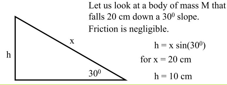
The kinetic energy at the bottom of the slope,  $E_{kin}(x)$  equals the kinetic energy after a free fall of height h,  $E_{kin}(h)$
