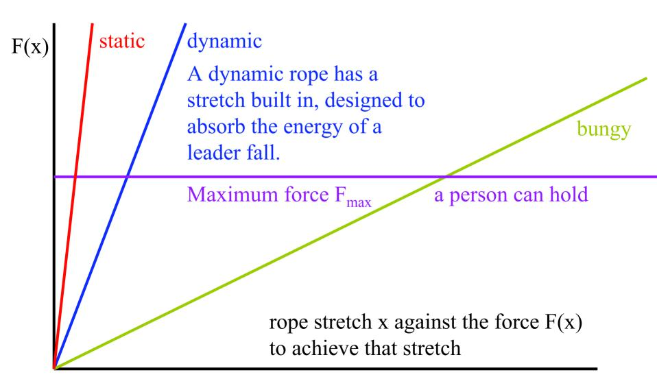
The area under the graph corresponds to the energy absorbed due to rope stretch.
