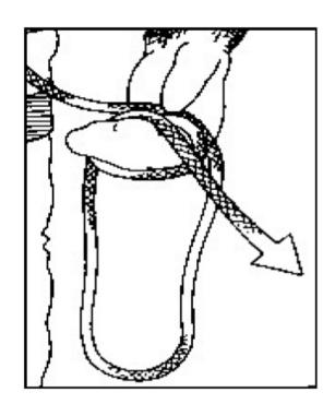
Dynamic hand brake for controlled slippage of rope.
