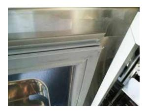
2. Peel back the existing door seal from one corner. This will reveal a groove that the door seal fits in.
