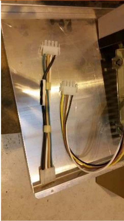
Cable connectors at the rear of the ice-maker cabinet.
