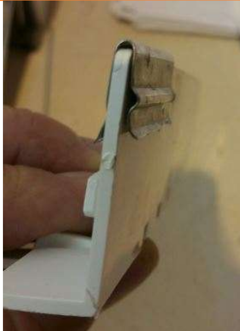
Thermostat sensor retaining clip.
