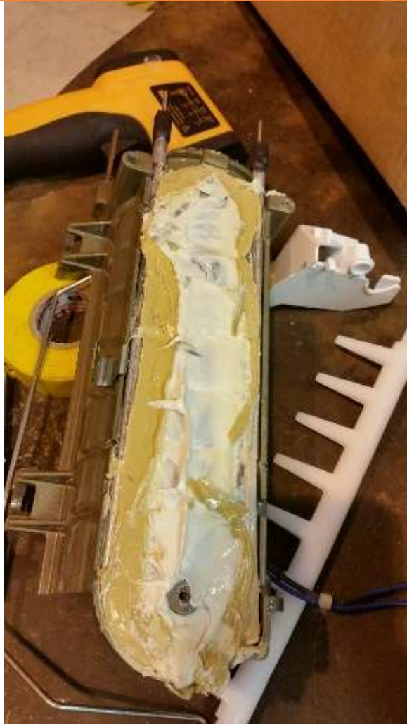
Thermal paste on the underside of the removed mechanism.
