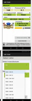
After clicking on the blue **Select Type** line, the list of valves of the given manufacturer will open. Select the required valve type. For simpler orientation and selection, also the picture for each valve type will be displayed for you.
