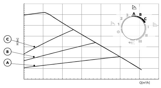
Proportional pressure functional mode is recommended in systems with relatively large pressure losses in the distribution pipes such as **radiator heating loops**.
