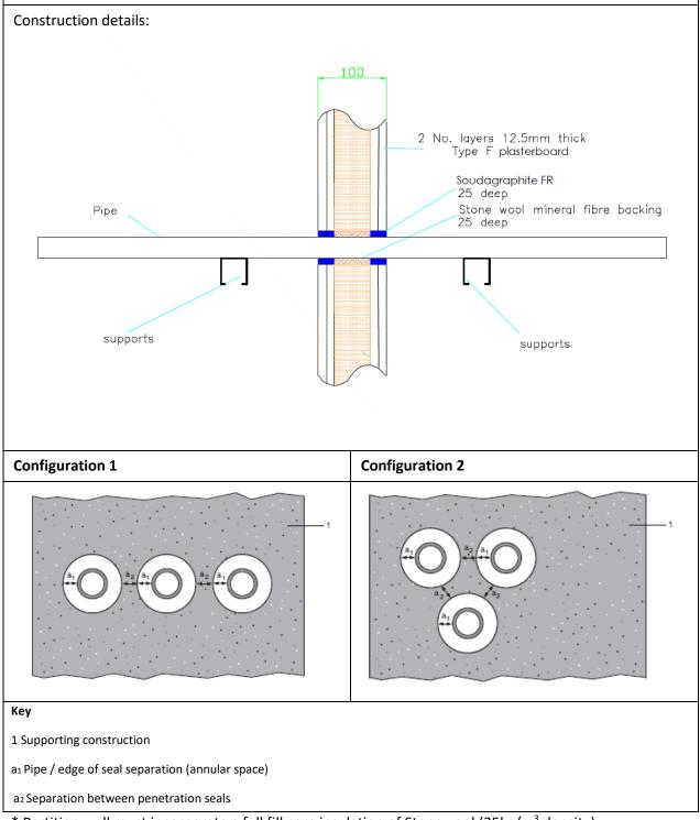
\* Partition wall must incorporate a full fill core insulation of Stonewool (35kg/m<sup>3</sup> density)
