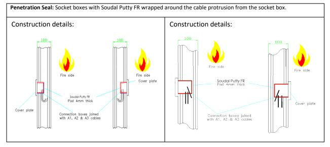
A.1.2.1 Single side penetration seal with cables in socket boxes
