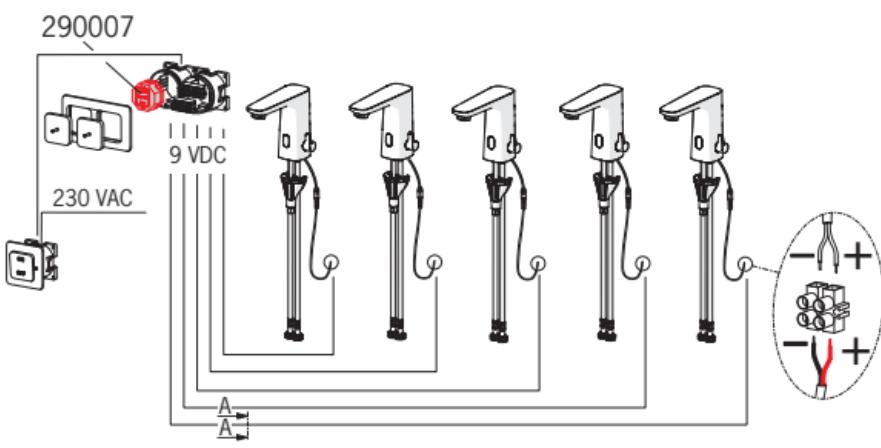
$2 \times \geq 0.5 \text{ mm}^2$
