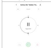
When Danfoss Ally™ is turned down to Min level manually, a notification banner is shown, and center icon switches to 'Pause'.
