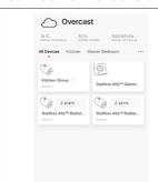
If several Radiator thermostats are assigned to one room the Danfoss Ally<sup>™</sup> App will automatically create a group. This is to ensure settings are synchronized between devices in same room. It is recommended to always adjust schedule and preferred temperatures from the group to ensure the most efficient performance.
