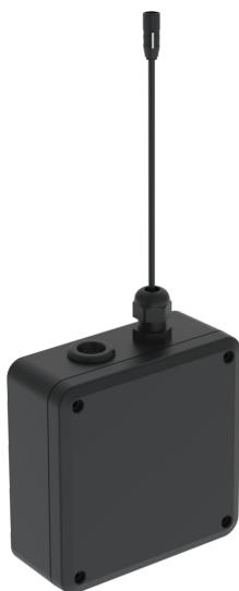
The power supply is designed for use with Electra products (9 V). A maximum 5 of these items can be connected to the power supply at a time (1 item is recommended). The total length of the cable between the power supply and the faucet may not exceed 50 m. Low-voltage cable  $2 \times >= 0.5 \text{ mm}^2$ . The transformer is installed in a 122x122 mm water tight box.
