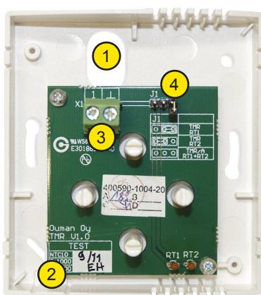
The room sensor can be mounted to the wall or on the top of a connection box. The case has holes on the bottom for both wall and box mounting.
