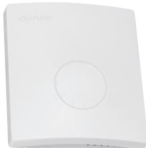
TMR sensor is placed at the height of approximately 150 cm in a place where it measures the mean temperature of the premises. Do not place the room sensor on direct sunlight or close to a heat source. The room sensor can be mounted to the wall or on the top of a connection box. This room sensor can also be used in measuring the average room temperature. Average value measurement is taken into use with the J1 jumper.
