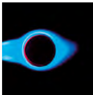
High flame temperature based on cyclone swirl
