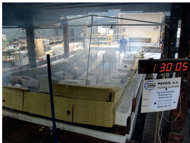
Figure 11. Sample after 90 minutes – roof deformation protected with ISOVER FireProtect® is close to limit deformation given by test standard EN 1365-2 (fluent transition from bending stress to membrane)
