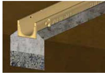
2. Connect pipe connections to the pipeline and align the components evenly.
