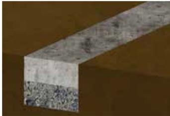
3. Fill concrete, 3 parts sand + 1 part water + 1 part cement, into the base of the trench.
