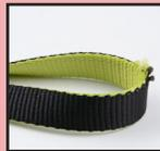
Tape edge damaged; numerous loops pulled
