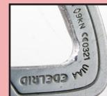
Significant material abrasion  $\geq 20\%$
