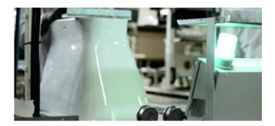
The pieces leaving the kiln are sent to the inspection and control area, where the defective pieces are separated from the conforming ones. Those that pass the final inspection are packed up and palletized for their transport to the dispatch warehouse. The complete cycle for the manufacturing of sanitary ware lasts approximately two to three days.
