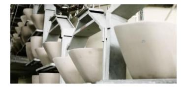
Once the piece has achieved a mechanical consistency within the plaster mould, it is removed manually or automatically, depending on the line or its difficulty. These pieces are placed on trolleys and transported to the different dryers, where they are dried with hot air. Once dry, they are transported again by trolleys, this time to the polishing and enameling line.
