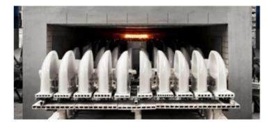
The enamelled pieces are then transported to the kiln area for their firing. The process of heating, firing, enamel vitrification and cooling takes place inside the kiln.
