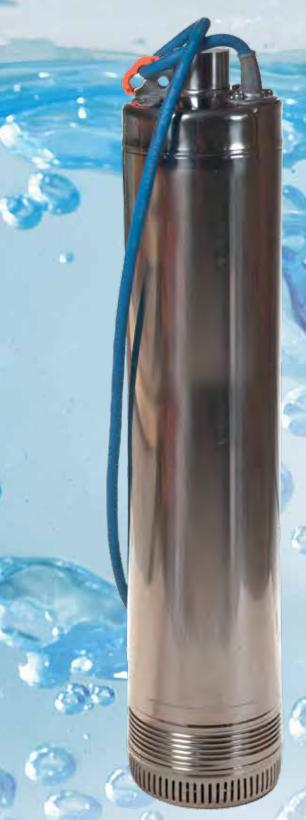
RIVER S pumps are intended for pumping household water from a dug well or basin. The electric cable is of Aqua quality. Water flows along the motor casing and cools the motor efficiently. The pump is equipped with an automatic air release valve, ensuring good operational reliability. The pump is made of stainless steel for improved operational reliability and increased performance. Dual mechanical seals increase lifespan and operational reliability.
