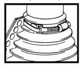
Insert hook into other band slot, and flatten with thumb forming clamp. Tighten screw with screwdriver to desired tension. Clamp is complete.
