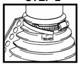
Bend end of band toward underside to form hook and insert in band slot on housing. Wrap the assembly snugly around object and at point ONE INCH BEYOND first serration, cut, then bend a 1"hook toward underside of band.
