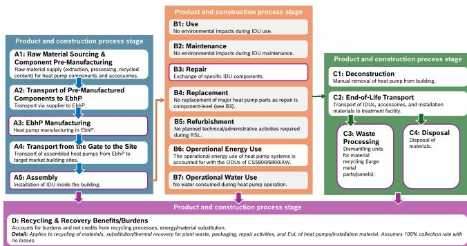
**Module A1-A3:** Raw material supply (extraction, processing, and recycled content) for the components the heat pump units comprise. This includes transport from raw material extraction to the supplier and from the supplier to the Bosch plant. Manufacturing processes at the Bosch plant are also covered, considering energy use, required consumables, production waste and its treatment, as well as internal transport.
