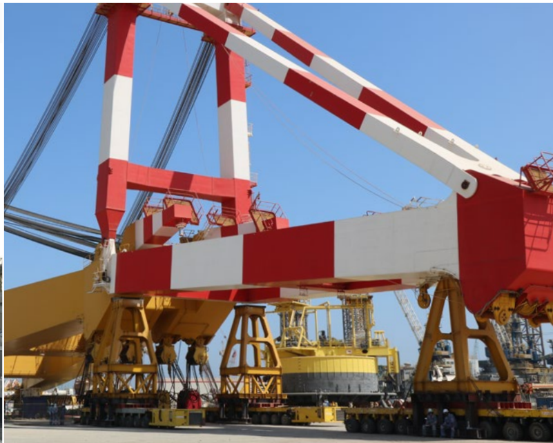
SEVEN INAGHA – MODIFICATION AND UPGRADATION WORK ASIAN HERCULES 3 – REMOVAL OF 200T FLY JIB
