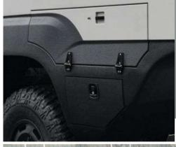
the world how a composite cabin specifically tailored to the Iveco Daily 4x4 chassis looks like. The cabin's body lines are matched perfectly for an integrated appearance. Its distinctive paint job consists of the upper half being in client-specific body color, while the lower half is coated in extremely resilient Raptor. All windows and outside storage hatches are molded flush with the cabin's surface in full carbon fiber frames.
