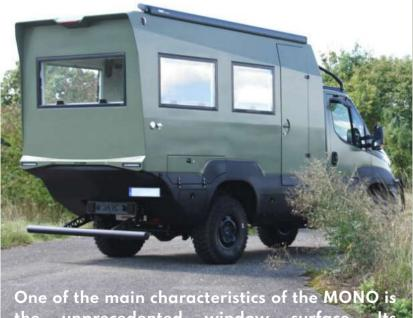
One of the main characteristics of the MONO is the unprecedented window surface. Its windows include one 1500x600mm (dining), two 1100x600mm (dining), one 900x600mm (kitchen) and one 600x350mm (bathroom). All of them can be opened, locked in ventilation mode, have bug meshes and 100% dark blinds. The skylights are 1500x600mm and 350x600mm in size. Check page 25 for more!
