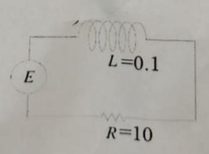
if the applied voltage is given as  $f(t) = \begin{cases} 0, & t \le 5 \\ 2, & t > 5 \end{cases}$ . Assuming the initial charge and voltage to be zero, compute the current at any time t using Laplace transform method. (Use the mathematical model Lq'' + Rq' + q/c = f(t)) (10 M)
