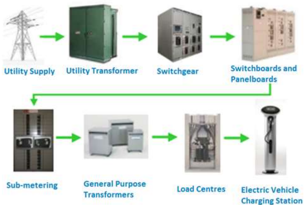
Fig. Components used in Charging Station
