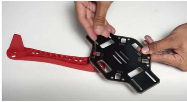
Fig 12.1 Drone Frame Assembly
