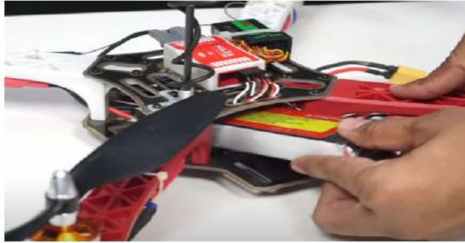
Fig 12.6 Inspection of Drone Wiring and Component Integrity & Power Supply Integration
