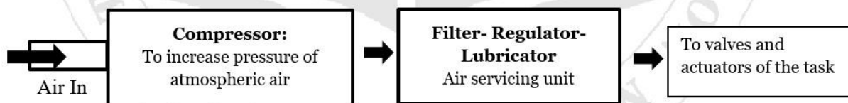
Fig.4.1 Role of Compressor and FRL unit in pneumatics
