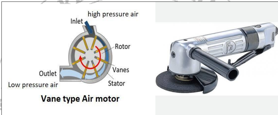
Fig.6.3 Vane type and turbine type Air motor
