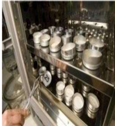
Containers in oven
