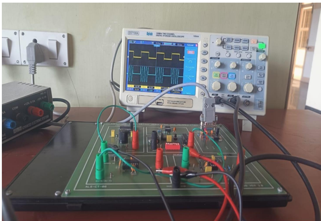
Figure 15.4: Practical set up for ASK modulation
