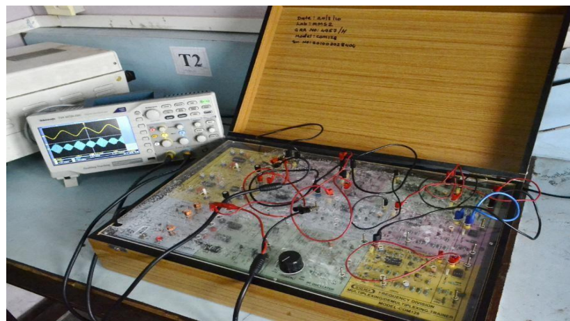
Figure 22.4: Practical set up for FDM system
