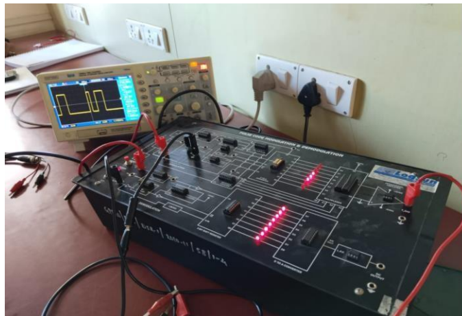
Figure 11.3: Practical set up for PCM
