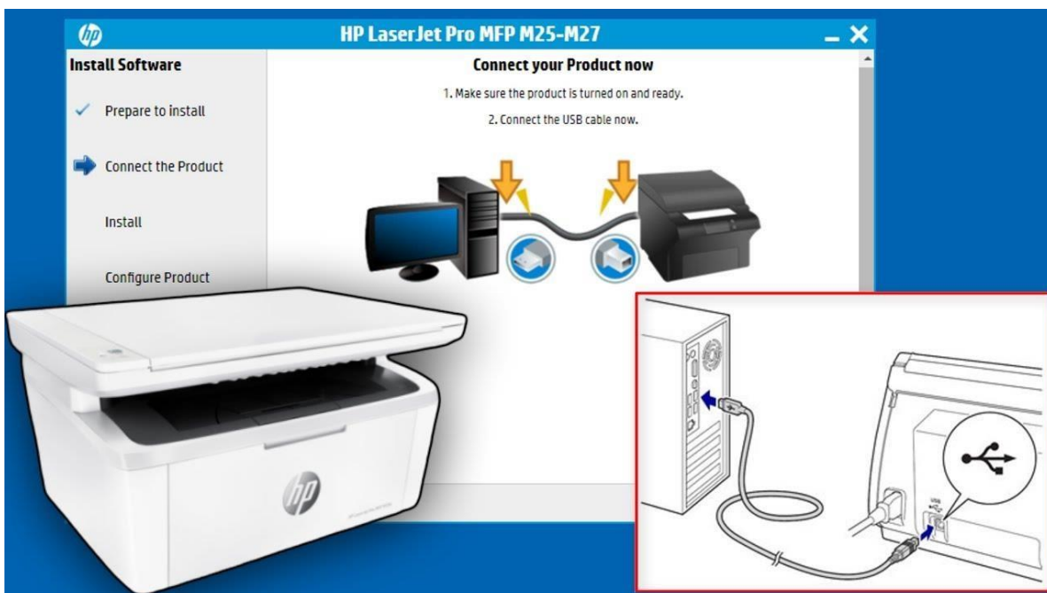
Figure 24.1. Laser printer connection diagram with Personal Computer.
