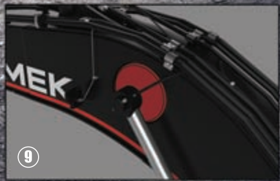
REINFORCED BOOM HYDRAULIC CYLINDER BEARING
