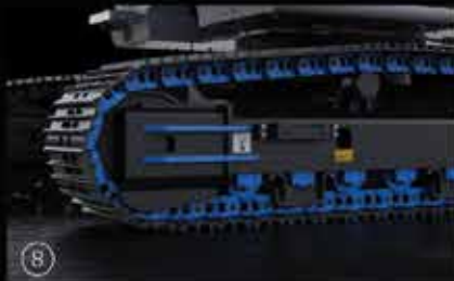
Reinforced lowerframe and undercarriage components
