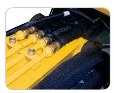
> Hydraulic hoses pass in the center of the upper frame: perfect protection and no twisting.
