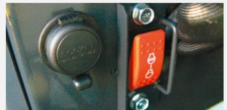
Electric engine stop (emergency stop)
