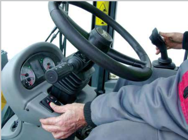
Electrical proportional adjustment of the hydraulic performance of the 3 rd circuit.
