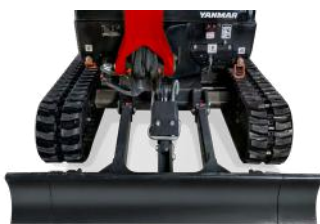
Extended undercarriage: 1170 mm
