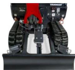
Retracted undercarriage : 980 mm
