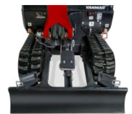
Retracted undercarriage : 980 mm
