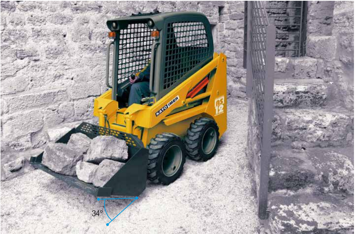
The bigger bucket rollback avoids material waste during transportation
