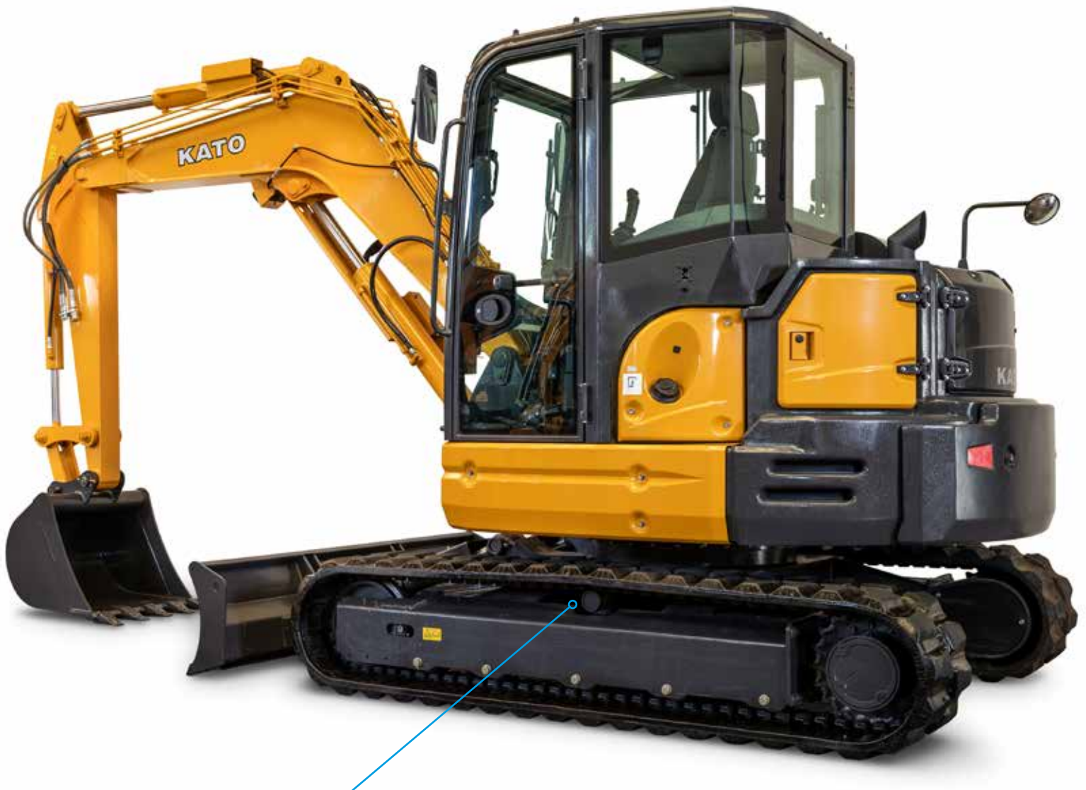
The crawler shoes pre-tensioning system is oversized and the guide roller has been positioned further back
