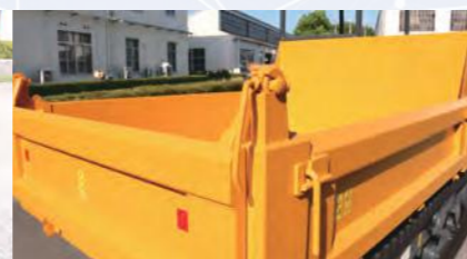
▲Sloped vessel frame
