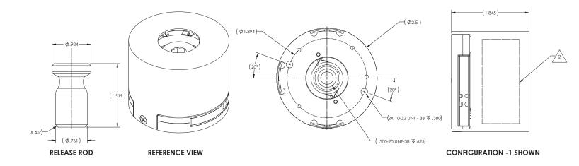
Note: Model 9104 Release Mechanism shown. Different configurations available with alternate release rods, mounting features, and connectors. Metric configurations are also available.
