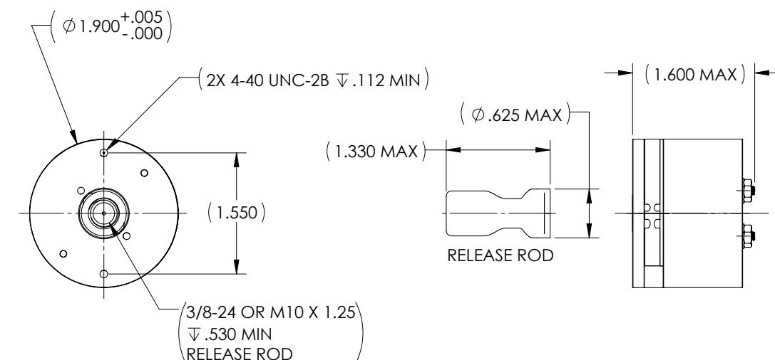
*Note: Model 9103 Release Mechanism shown. Different configurations available with alternate release rods, mounting features, and connectors. Metric configurations are also available.*
